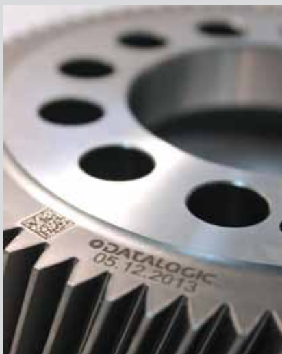
High contrast marking on metal
